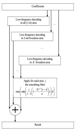
Figure 3: Scheme of foveation-decoding
